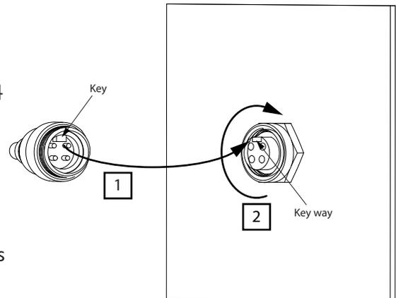
To remove, unscrew the connector fully and pull out of the receptacle.
