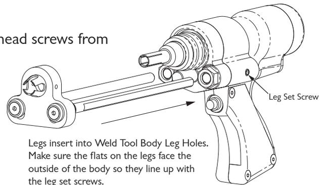
Legs insert into Weld Tool Body Leg Holes. Make sure the flats on the legs face the outside of the body so they line up with the leg set screws.
