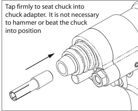
To install a chuck, position the chuck into the front of the chuck adapter. Tap lightly on the end to seat the chuck into the adapter. It is not necessary to pound on the end of the chuck. This will only damage the chuck itself.
