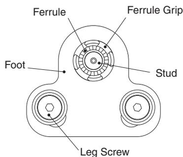
Alignment of the foot is very important, if the foot is not aligned properly it can create bad welds in the form of hang-ups. Place a stud into the chuck and a ferrule into the ferrule grip. The stud should sit perfectly in the center of the ferrule. If it does not, loosen the flat head screws on the legs holding the foot. Position the foot so the stud is perfectly aligned in the ferrule. Retighten the flat head screws.
